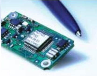
*The AD105 is a very compact printed circuit board which can be integrated into your load cells. Alternatively, it can be mounted on one side of the load cell and covered with a shield cap (available from HBM).*
